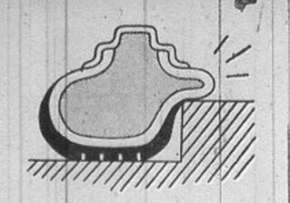
Rough-riding over pavement curbs and bad roads damages tyre covers. Drive carefully, and remember the cardinal rule of tyre preservation—always keep your tyres inflated to the recommended air pressure.
