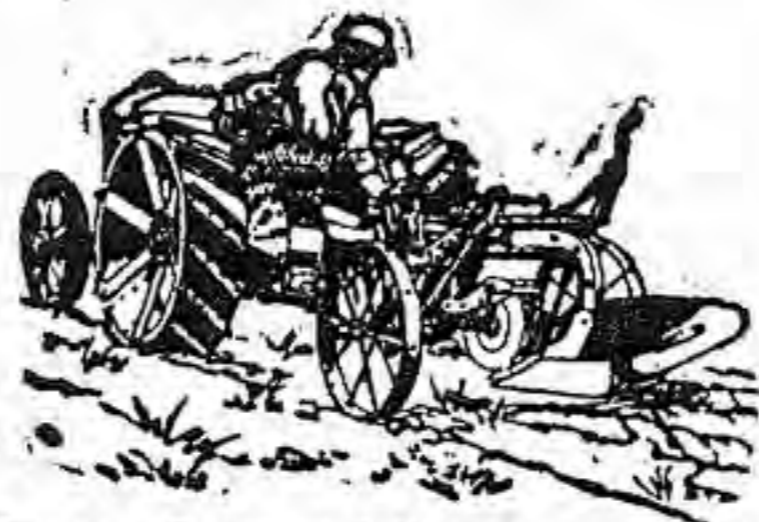
FORDSON TRACTOR delivered to purchaser. 22 horse power, 3 speed and reverse, weight 25 cwt., length 8ft 6in, width 5ft 2in. Height 4ft 4in. Price (at Works, Cork), £225. Extra for pulley attachment £10 10s 0d. Road bands for wheels £8 0s 0d.
